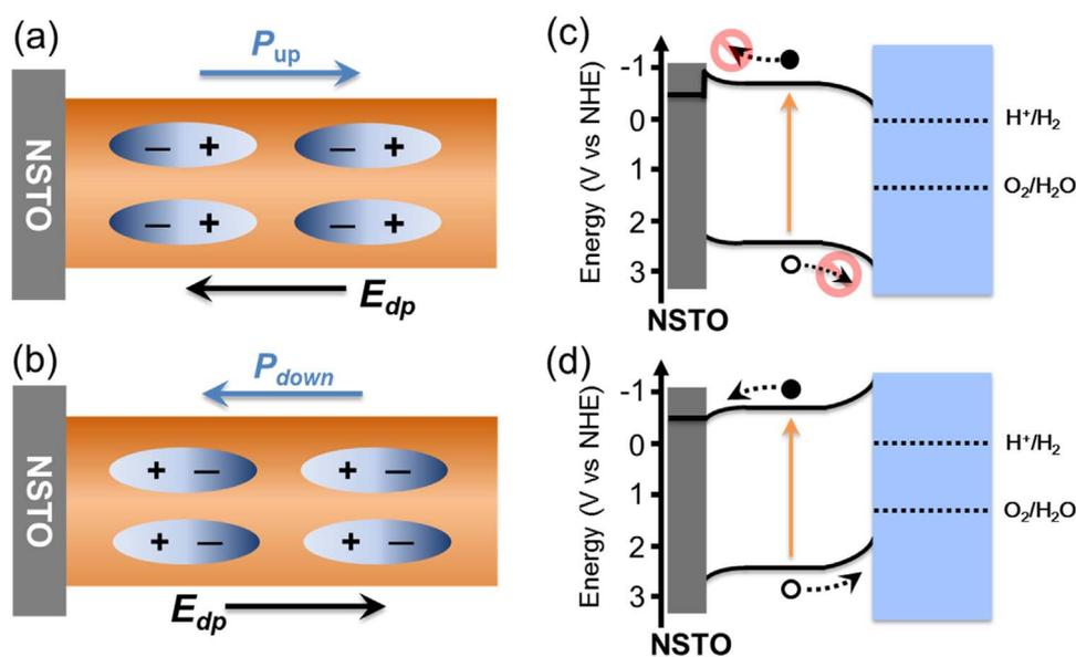
**Fig. 5.** A schematic diagram showing polarization bound charge under two different oriented polarization conditions: (a) positively and (b) negatively poled KNO NW arrays. *P* is the polarization, and *E<sub>dp</sub>* is the depolarization field. (c and d) Proposed electronic band structure and the mechanisms for the charge transfer process in the KNO NW array photoelectrodes for the two poling configurations.
