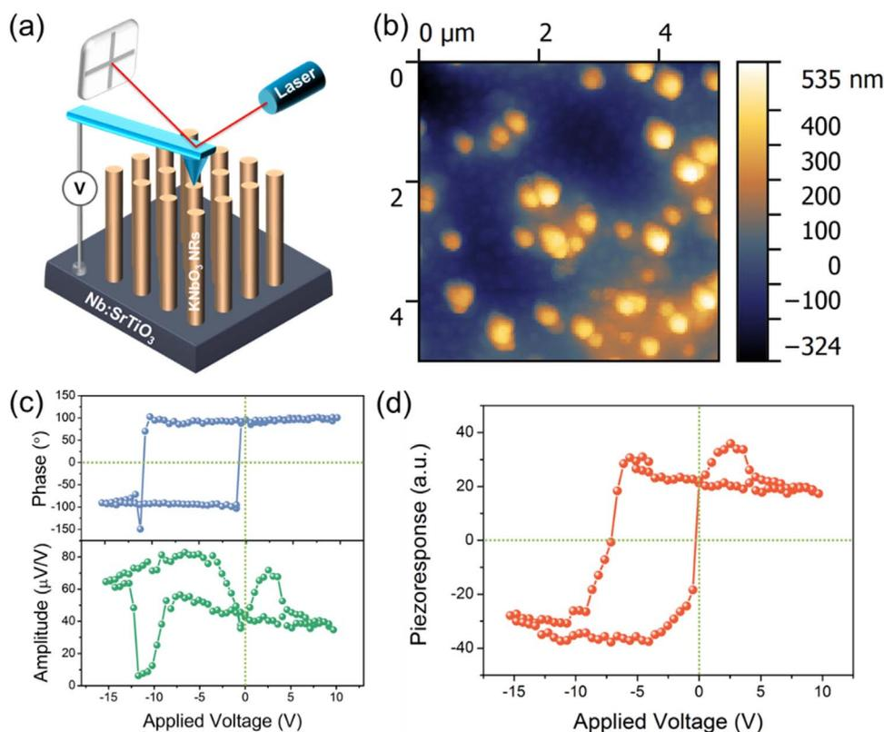
**Fig. 3.** (a) Schematic illustration of PFM measurement on a single KNO NW. (b) AFM topography image showing the surface of the NW arrays. DC bias induced local PFM (c) phase signal and piezoelectric strain amplitude, and (d) piezoresponse curve of a single KNO NW.
