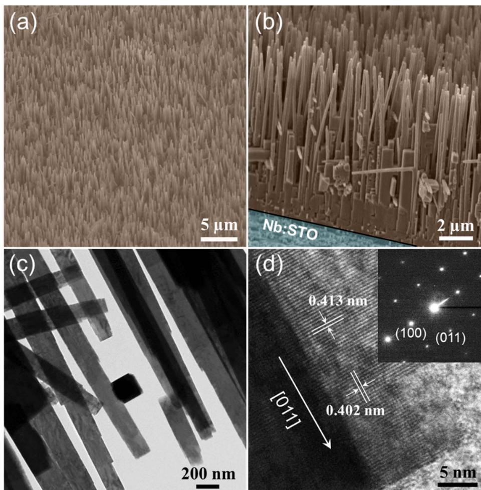
**Fig. 1.** (a, b) SEM images of KNO NW arrays epitaxially grown on NSTO (100) substrate. (c) Low-magnification TEM and (d) HR-TEM image of the KNO NWs. SAED patterns are shown in the inset of (d).
