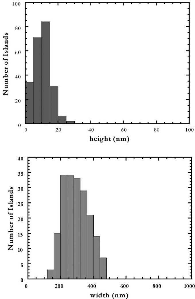
Fig. 3. Histograms of the islands height (left) and width (right) for a sample grown at 550 °C and with a total deposition of 2.0 nm Ge.
