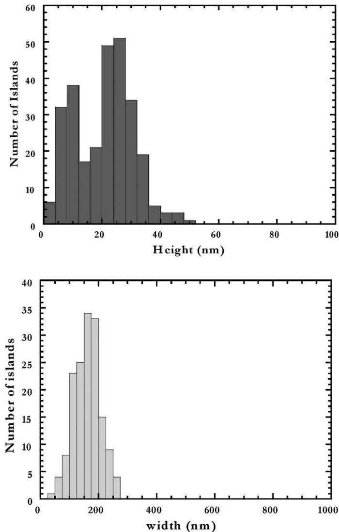
Fig. 2. Histograms of the islands height (left) and width (right) for a sample grown at 450 °C and with a total deposition of 2.5 nm Ge.
