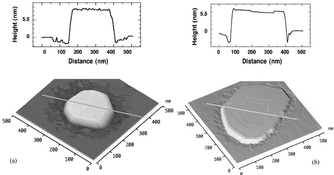
Fig. 1. Ge/Si(1 1 1): (a)  $527 \times 527 \text{ nm}^2$  STM image of an island at the first stage of ripening (3.5 nm of Ge/Si(1 1 1) at  $T = 500 \text{ }^\circ\text{C}$ )—island height: 10 nm. (b)  $527 \times 527 \text{ nm}^2$  AFM image in the gradient mode of an island transformed in atoll at the final stage (2 nm of Ge/Si(1 1 1) at  $T = 500 \text{ }^\circ\text{C}$ )—island height: 8 nm.
