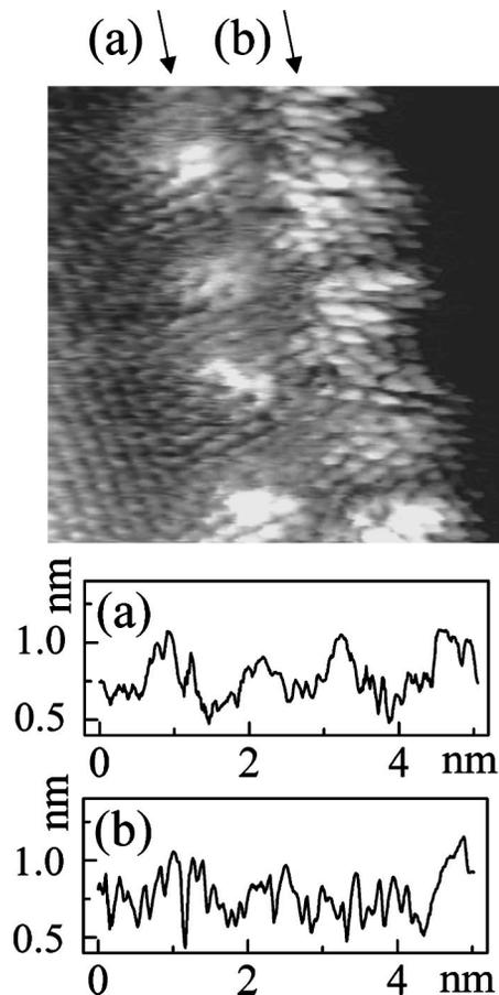
FIG. 2. STM image ( $5 \times 5 \text{ nm}^2$ ) of two coiled adjacent nanotubes ( $I_t = 1 \text{ nA}$  and  $V_t = 0.1 \text{ V}$ ). The lower panel shows the line profiles obtained along the directions indicated by the arrows (a) and (b), respectively.
