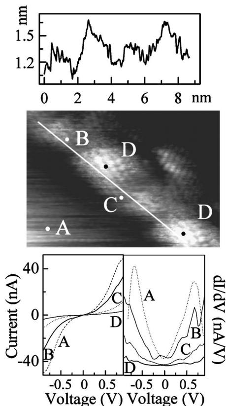
FIG. 3. STM image ( $5 \times 5 \text{ nm}^2$ ) showing two coiled nanotubes twisted together. The upper panel shows the line profile along the white line drawn on the STM image. The lower panels show the  $I$ - $V$  curves recorded around points A, B, C, and D, respectively, and the corresponding  $dI/dV$  curves obtained by differentiation.
