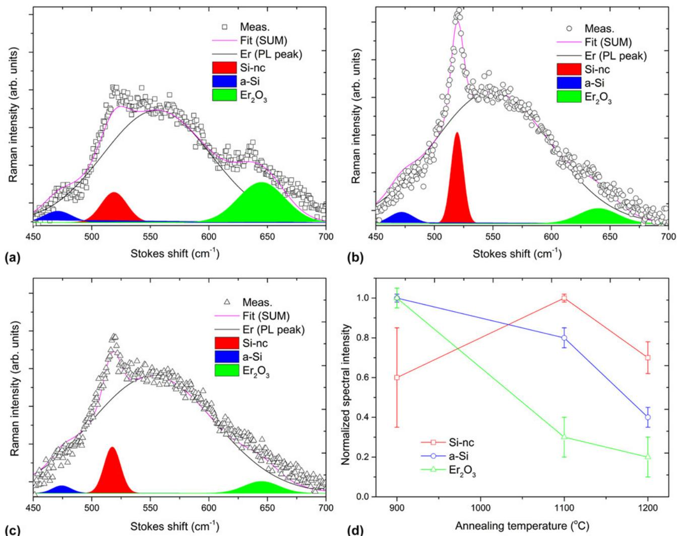
FIG. 4. Raman analysis of zone-2 samples at different annealing temperatures (a) 900 °C, (b) 1100 °C and (c) 1200 °C. (d) The graph representing the relative variations of phases present at different annealing temperatures.
