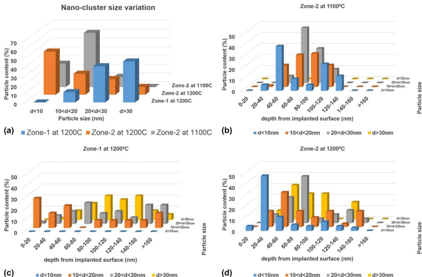
FIG. 6. (a) Er nanoparticle size variations and the in-depth size distribution analysis for (b) zone-2 at 1100 °C, (c) zone-1 at 1200 °C, and (d) zone-2 at 1200 °C.
