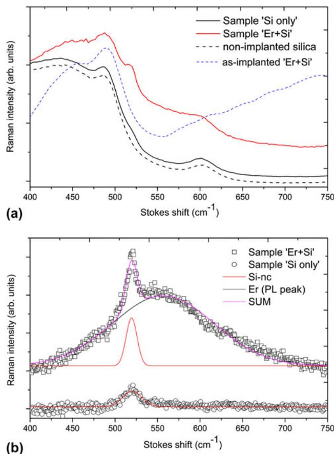
FIG. 2. The comparison of Si-nc peaks in Raman spectra obtained from zone-2 (top) and zone-3 (bottom) samples annealed at  $1100\text{ °C}$ , before (a) and after (b) removing the contribution of fused silica.
