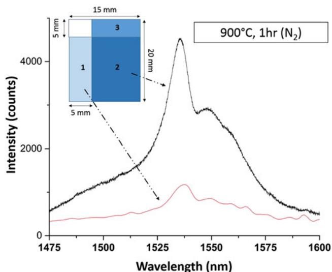
FIG. 1. PL-NIR spectra exhibiting comparison of Er 4f-shell emission (<sup>4</sup>I<sub>13/2</sub> → <sup>4</sup>I<sub>15/2</sub>) between zone 1) Er<sup>3+</sup> and 2) Si<sup>+</sup> and Er<sup>3+</sup> (designation of different implantation zones on amorphous SiO<sub>2</sub> is shown in figure inset; 1) Er<sup>3+</sup>, 2) Si<sup>+</sup> and Er<sup>3+</sup>, 3) Si<sup>+</sup>).
