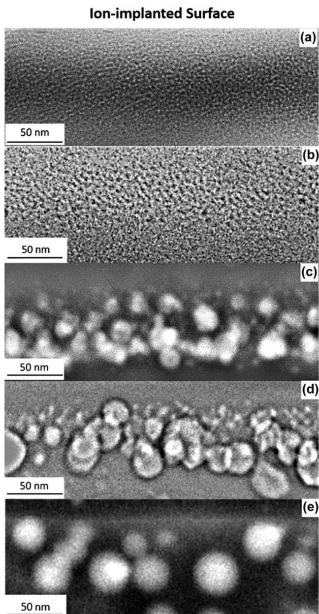
FIG. 5. TEM and S/TEM images of ion-implanted regions of different zones; (a) zone-1 ( $\text{Er}^{3+}$ ) as-implanted, (b) zone-3 ( $\text{Si}^+$ ) at 1100 °C, (c) zone-2 ( $\text{Si}^+$  and  $\text{Er}^{3+}$ ) at 1100 °C, (d) zone-2 ( $\text{Si}^+$  and  $\text{Er}^{3+}$ ) at 1200 °C, and (e) zone-1 ( $\text{Er}^{3+}$ ) at 1200 °C.
