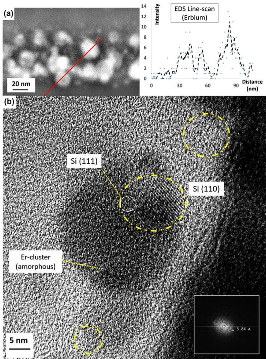
FIG. 3. (a) The EDS line-scan of Er-np in zone-2 samples annealed at 1100 °C for 1 h under N<sub>2</sub> atmosphere and (b) TEM BFI showing the presence of Si-nc (with fast Fourier transform [FFT] shown at the bottom right corner) in the vicinity of amorphous Er-np.
