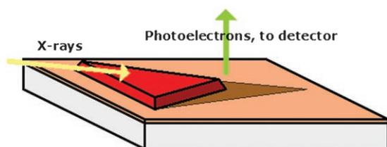
**Figure 3.** Scheme of a Ge(Si) nanostructure with a morphology typical of those observed on the Ge/Si(111) surface. The X-ray flux (yellow arrow) impinges the sample in a grazing configuration. Photoelectrons (green arrow) are collected from the normal direction. Outstanding features include the X-rays' shadows on specific steep facets of the islands and areas of the WL. Note however that the top-most (111)-oriented facet of the nanostructures is always completely illuminated.
