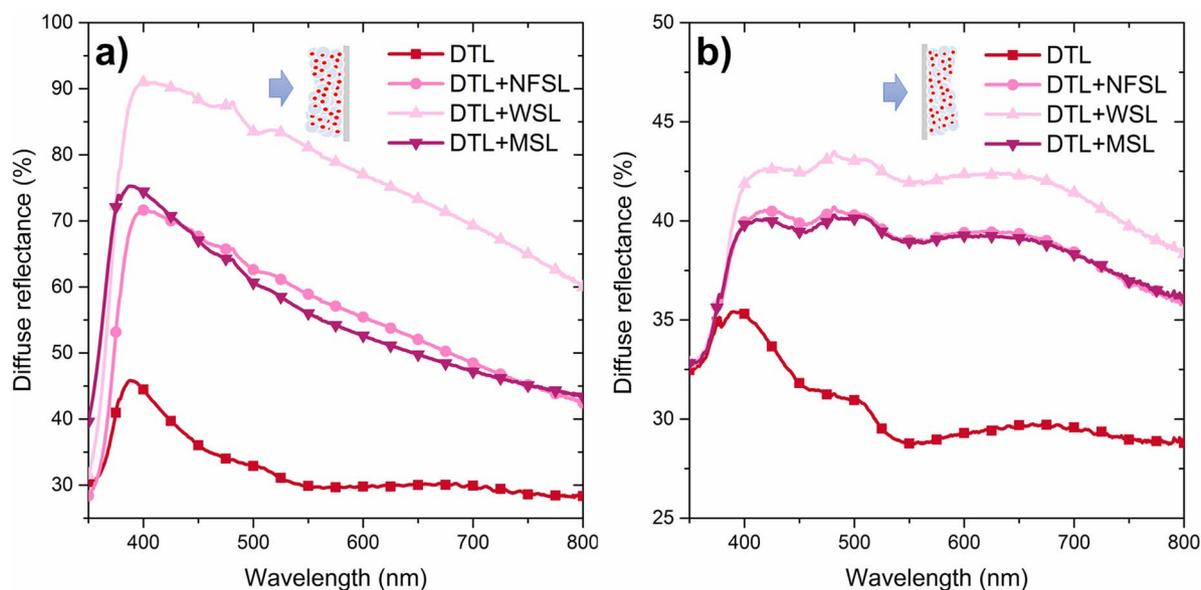
**Figure 5.** Diffuse reflectance spectra measured under (a) front and (b) rear illumination.
