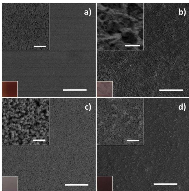
**Figure 3.** SEM and digital images of the photoanodes. (a) DTL, (b) NFSL (c) WSL and (d) MSL. SEM scale bar: 10  $\mu\text{m}$  in low magnification images and 1  $\mu\text{m}$  in top insets. The lower insets represent the photoanode after sensitization, square dimension: 25  $\times$  25  $\text{mm}^2$ .
