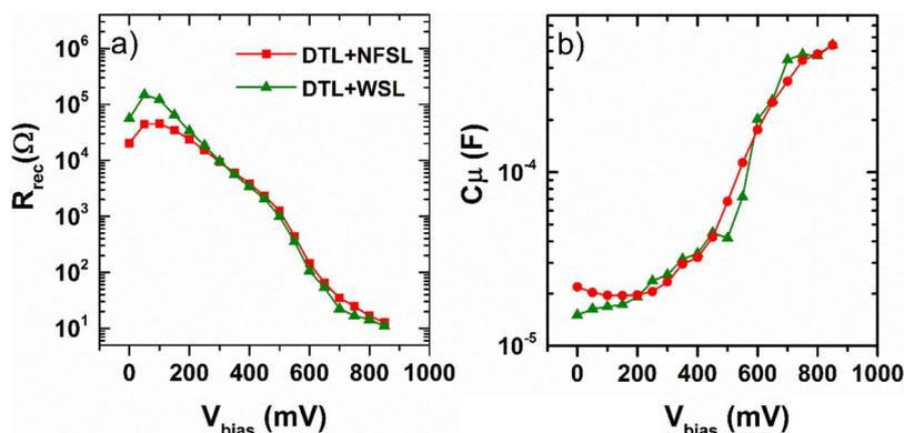
**Figure 6.** EIS analysis of DSSCs with different scattering layers. (a) Recombination resistance and (b) chemical capacitance from EIS measurements in dark.
