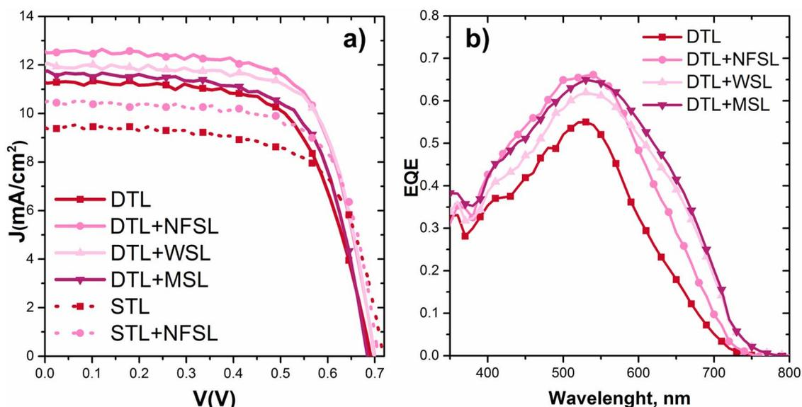
**Figure 4.** (a)  $J$ - $V$  curves of DSSCs with different photoanodes. (b) EQE spectra of DSSCs with different structured photoanodes.
