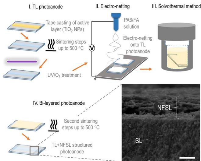
**Figure 1.** Scheme showing the bi-layered photoanode preparation steps and STL + NFSL cross section. SEM scale bar equals 2  $\mu\text{m}$ .
