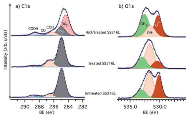
Fig. 5 XPS spectra of (a) C 1s, and (b) O 1s on untreated SS316L, treated SS316L and rGO/SS.
