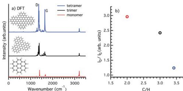
Fig. 4 (a) Calculated Raman spectra for each DFT optimized structures (single-coronene, trimer-coronene and tetramer-coronene). (b) Carbon–Hydrogen (C/H) vs.  $I_D/I_G$  ratios.
