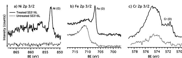
Fig. 1 XPS spectra of Ni 2p<sub>3/2</sub>, Fe 2p<sub>3/2</sub>, Cr 2p<sub>3/2</sub> for untreated SS316L (below) and treated SS316L (above).
