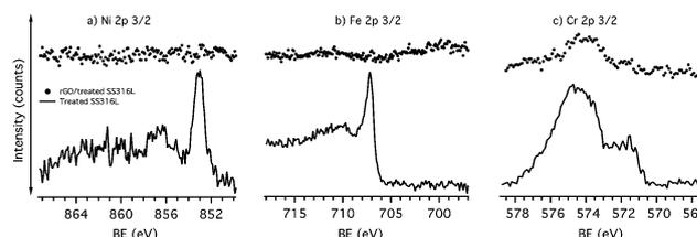
Fig. 6 XPS spectra of Ni 2p<sub>3/2</sub>, Fe 2p<sub>3/2</sub>, Cr 2p<sub>3/2</sub> for treated SS316L (below) and rGO/treated SS316L (above).
