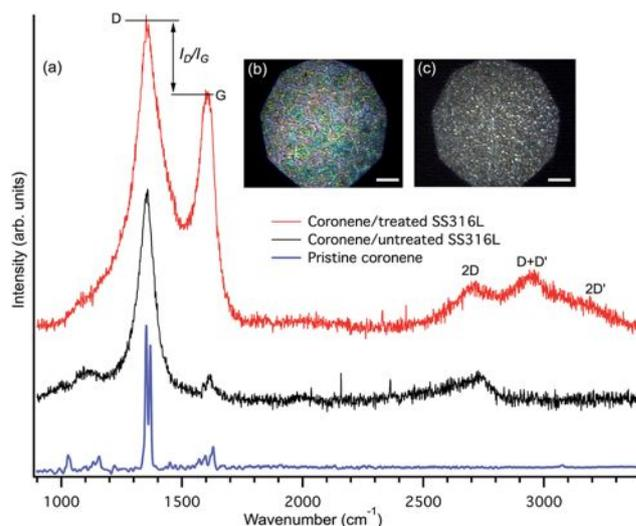
Fig. 2 (a) Raman spectra corresponding to rGO (red curve), coronene on untreated SS316L (black curve) and coronene on glass (blue curve) on the same area where optical images were taken for: (b) rGO/SS316L and (c) coronene/untreated SS316L. Scale bars in the inset images represent 20  $\mu m$ .
