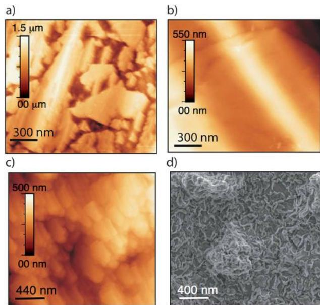
Fig. 3 AFM images on untreated SS316L (a), treated SS316L (b) and rGO/SS316L (c). SEM image on rGO/SS316L (d).
