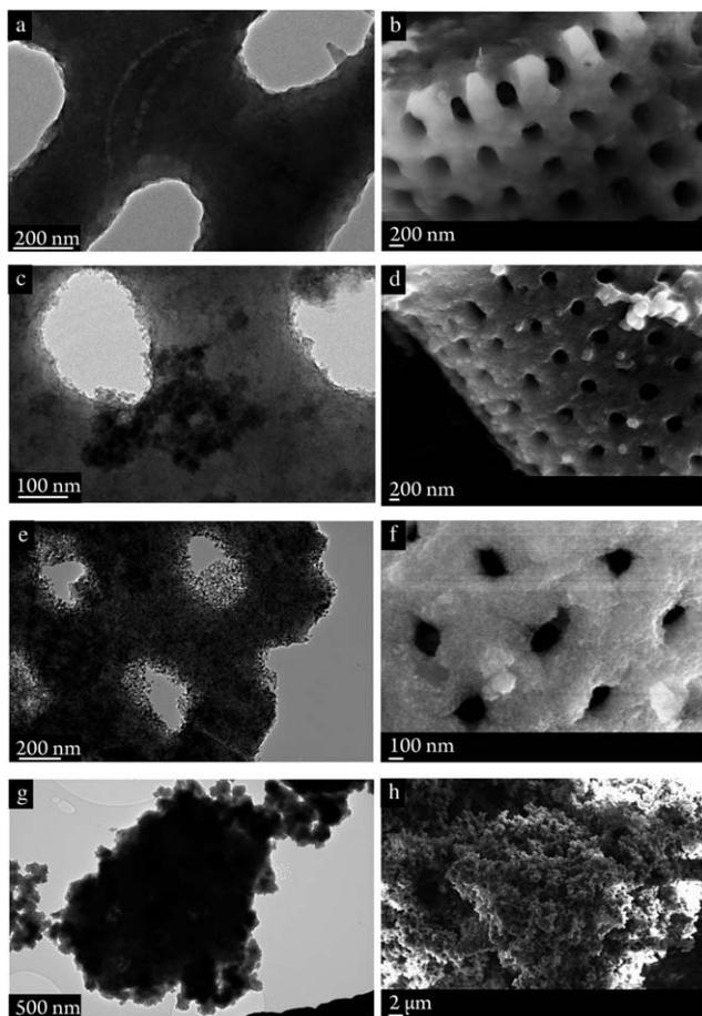
**Fig. 2** TEM (left) and SEM (right) of pristine diatoms (a and b) and titania coated diatoms after 1 cycle (c and d), 2 cycles (e and f) and 3 cycles (g and h).
