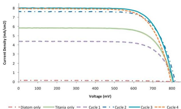
**Fig. 3**  $I$ - $V$  curves for diatom only, titania only and titania coated diatoms, cycles 1-4.
