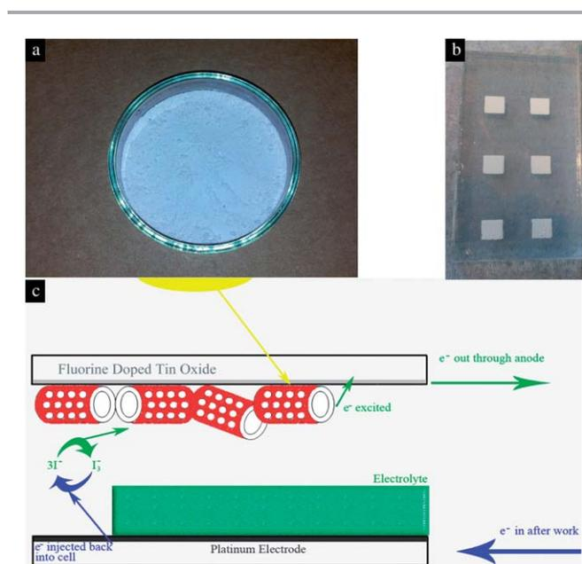
**Fig. 1** Image of diatomaceous earth (a) and the working electrode made by screen printing the diatom paste (b). Schematic of the DSSC incorporating diatomaceous earth (c).
