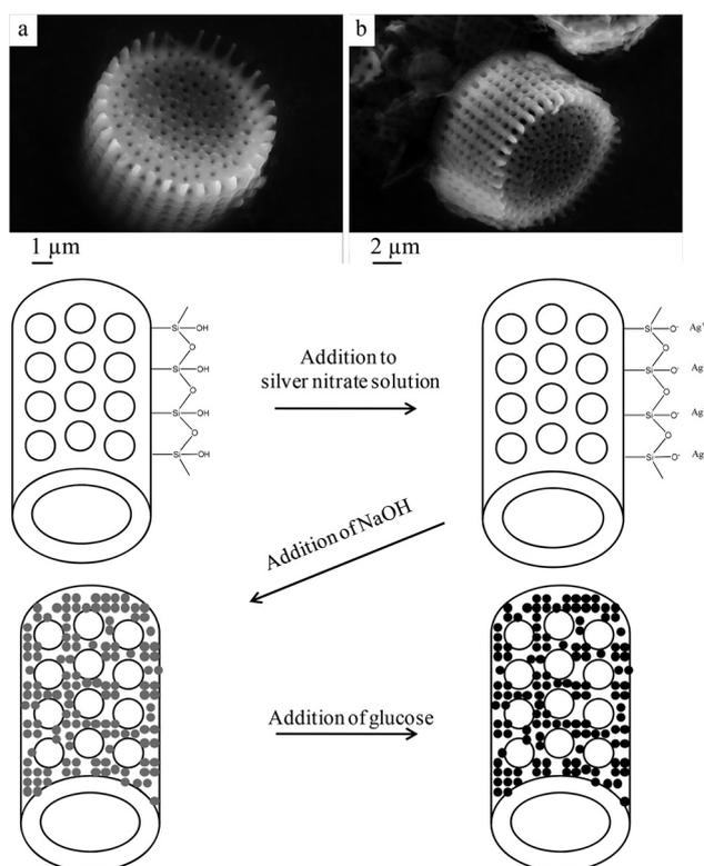
**Fig. 1** Scanning electron microscope (SEM) images of diatom frustules after plasma etching (a and b) along with coating procedure schematic for plasma treated frustules being added to 4 mL 0.005 M  $\text{AgNO}_3$ , then the addition of 70  $\mu\text{L}$  0.5 M NaOH and finally the addition of 500 mg of glucose.
