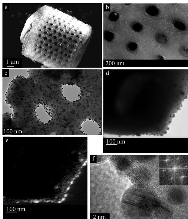
**Fig. 2** Low resolution SEM (a), high resolution SEM (b) and TEM (c) images of silver coated diatoms. TEM (d) image and corresponding energy filtered TEM (e) of silver coated diatoms, and high resolution TEM (f), with corresponding electron diffraction pattern.
