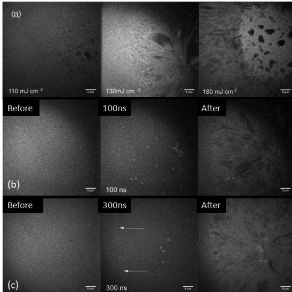
FIG. 3. Sequence of images of microstructure as function of the incident laser fluence (a) sequence of images for fluence of  $155 \text{ mJ cm}^{-2}$  at 100 ns and 300 ns time delays [(b) and (c)], respectively.
