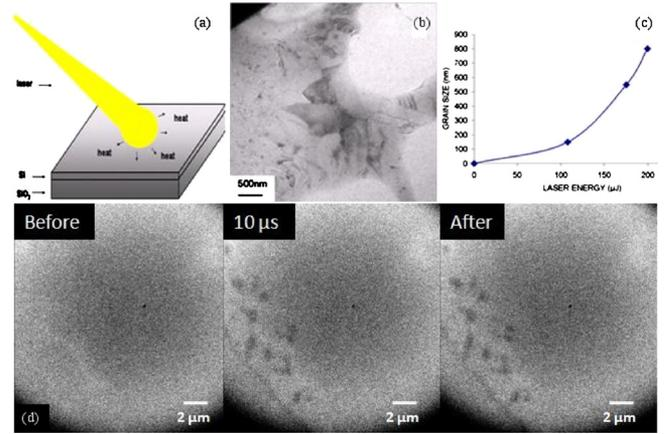
FIG. 2. (Color online) Schematic of drive laser incident on sample (a) cw electron beam images showing plan views of film shot at  $\sim 108$  and  $175.5 \mu\text{J}$  (b) Maximum grain size after crystallization experiment as a function of laser energy. (c) Grain size=approximate diameter of largest grain shown in field of view; and sequence of images of microstructure at  $10 \mu\text{s}$  time delay for a fluence of  $\sim 108 \mu\text{J}$  (d).
