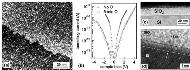
FIG. 1. (a) STM image ( $V_{\text{sample}}=3.5$  V) of a Si(100) surface after 5 min exposure to atomic O. (b) STS  $I$ - $V$  characteristics of clean Si(100) (crosses) and the same surface exposed to atomic O for 5 min (circles). The continuous lines are guides to the eye. [(c) and (d)] Cross-sectional bright field TEM micrographs of a 25-nm-thick oxide layer deposited at a growth rate of  $\sim 0.2$  nm/min.
