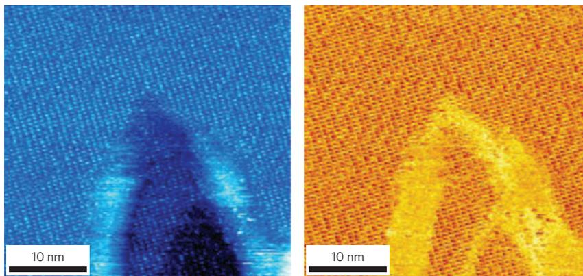
**Figure 1** | Mapping solid–liquid adhesion energy with an AFM. Small-amplitude-modulation atomic force microscopy images of calcite ( $\text{CaCO}_3$ ) in ultrapure water. A topographic image is shown in blue and a phase image, which maps the phase of the cantilever oscillation during a scan, is shown in yellow. (Figure courtesy of F. Stellacci).
