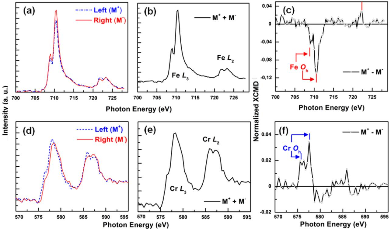
**Figure 3.** XPEEM local spectra for (a) Fe L-edges and (d) Cr L-edges. Corresponding XAS/XMCD spectra for Fe ((b)/(c)) and Cr ((e)/(f)). The XMCD intensities were normalized by the intensities of the XAS peaks.
