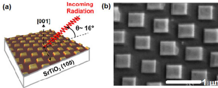
**Figure 1.** (a) AFM topography image of BFCO nanostructures grown on STO substrate and XPEEM experimental geometry. (b) SEM image showing the square shape of the submicron BFCO structures.
