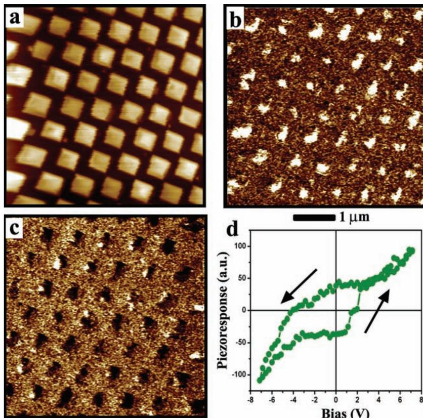
**Figure 3.** AFM/PFM measurements: a) Contact topography AFM image simultaneously recorded with the OP-PFM image (b) and IP-PFM (c). The z-range is 50 nm for topography; the z-scale for OP-PFM and IP-PFM images is in arbitrary units. d) Piezoresponse hysteresis loop recorded from an individual BFCO island in OP-PFM mode.
