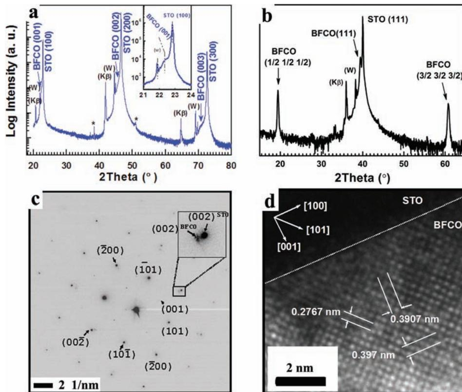
**Figure 2.** X-ray diffraction spectra of a) (001) and b) (111)-oriented BFCO nanostructures. c) Electron diffraction pattern of a 350 nm BFCO nanostructure along the [010] direction and d) high-resolution cross-section TEM image of the epitaxial BFCO layer taken along the [010] direction.
