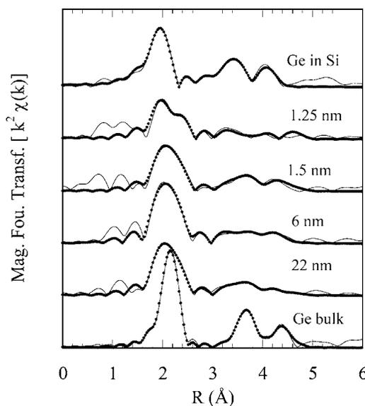
FIG. 4. Fourier transform of the XAFS spectra shown in Fig. 3 for selected samples around the Ge K-edge. Dots: Fourier transform of XAFS data. Lines: fitting.
