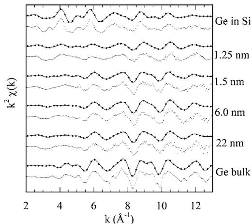
FIG. 3. XAFS spectra of selected samples around the Ge K-edge. For each sample the thickness of deposited Ge is indicated. Small dots: experimental data. Large dots: Fourier-filtered data. Lines: fitting.
