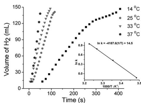
Fig. 5 – The volume of hydrogen versus time graph for the Ru/C catalytic hydrolysis of AB at different temperatures, [Ru] = 0.85 mM, [AB] = 200 mM. The inset shows the Arrhenius plot (ln *k* versus the reciprocal absolute temperature, 1/*T* (K<sup>-1</sup>)).
