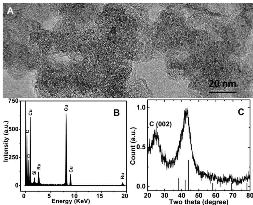
Fig. 1 – (A) TEM image of the Ru nanoclusters on the carbon black support. (B) EDX and (C) XRD pattern of the Ru/C catalysts.
