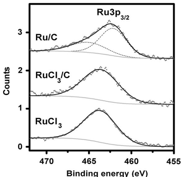
Fig. 2 – High resolution Ru 3p XPS spectra of filtered solutions of  $\text{RuCl}_3$ ,  $\text{RuCl}_3/\text{C}$  (after mixing  $\text{RuCl}_3$  with carbon black for 12 h), and  $\text{Ru}/\text{C}$  (after reducing  $\text{RuCl}_3$  by AB). The gray dots represent the experimental data. The black dash and gray solid lines are fitting and background curves, respectively. In the top spectrum, the black solid line is the sum of two black dash fitting curves.
