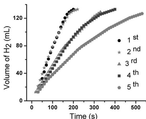
**Fig. 6 – Graph of hydrogen versus time for the Ru/C catalytic hydrolysis of AB from 1st to 5th cycles at  $22 \pm 1$  °C,  $[\text{Ru}] = 0.85$  mM, and  $[\text{AB}] = 200$  mM.**
