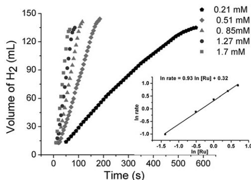
Fig. 4 – The volume of hydrogen versus time graph for the Ru/C catalytic hydrolysis of AB for different Ru concentration at 25 ± 1 °C. The inset shows the plot of hydrogen generation rate versus the concentration of Ru (both in logarithmic scale).
