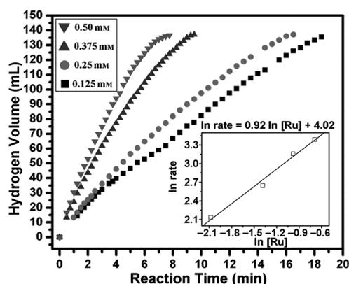
Figure 6. Plots of hydrogen evolution versus time during AB hydrolysis catalyzed by  $\text{Ni}_{0.74}\text{Ru}_{0.26}$  NPs at  $30 \pm 1^\circ\text{C}$  and at different catalyst concentrations. The inset shows the plot of hydrogen-generation rate versus catalyst concentration (both in logarithmic scales).
