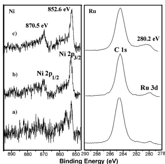
Figure 3. Left panel: Ni XPS spectra of the  $\text{Ni}_{0.74}\text{Ru}_{0.26}$  alloy NPs: a) before  $\text{Ar}^+$  ion sputter etching; b) after 2 min etching; c) after 5 min etching. Right panel: Ru XPS spectra of the  $\text{Ni}_{0.74}\text{Ru}_{0.26}$  alloy NPs in the same conditions as reported in the left panel.
