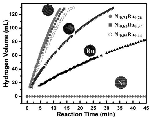
Figure 4. Comparison of catalytic activities of monometallic Ni, monometallic Ru, Ni@Ru core shell, and Ni–Ru alloy NPs for AB hydrolysis at  $30 \pm 1^\circ\text{C}$ .  $[\text{Ru}] = 0.25 \text{ mM}$  in monometallic Ru, in Ni@Ru, and in Ni–Ru alloy NPs; for monometallic Ni,  $[\text{Ni}] = 1 \text{ mM}$ ;  $[\text{AB}] = 200 \text{ mM}$ ; volume of the dispersion = 10 mL.
