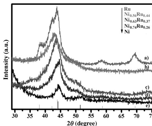
Figure 1. XRD patterns of pure a) Ru, b) Ni<sub>0.56</sub>Ru<sub>0.44</sub>, c) Ni<sub>0.63</sub>Ru<sub>0.37</sub>, d) Ni<sub>0.74</sub>Ru<sub>0.26</sub>, and e) pure Ni. Gray vertical lines represent the hcp Ru phase (JCPDS file 06-0663) and black vertical lines the fcc Ni phase (JCPDS file 04-0850).
