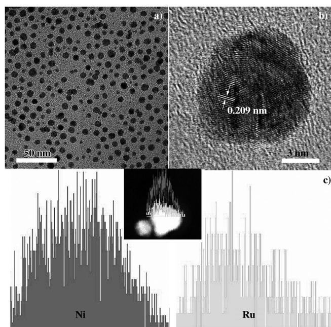
Figure 2. a) TEM image of a  $\text{Ni}_{0.74}\text{Ru}_{0.26}$  alloy NPs sample; b) HRTEM image of a single  $\text{Ni}_{0.74}\text{Ru}_{0.26}$  alloy NP; c) Ni and Ru compositional-line profiles recorded along the median line of a single particle in the STEM image (see inset).
