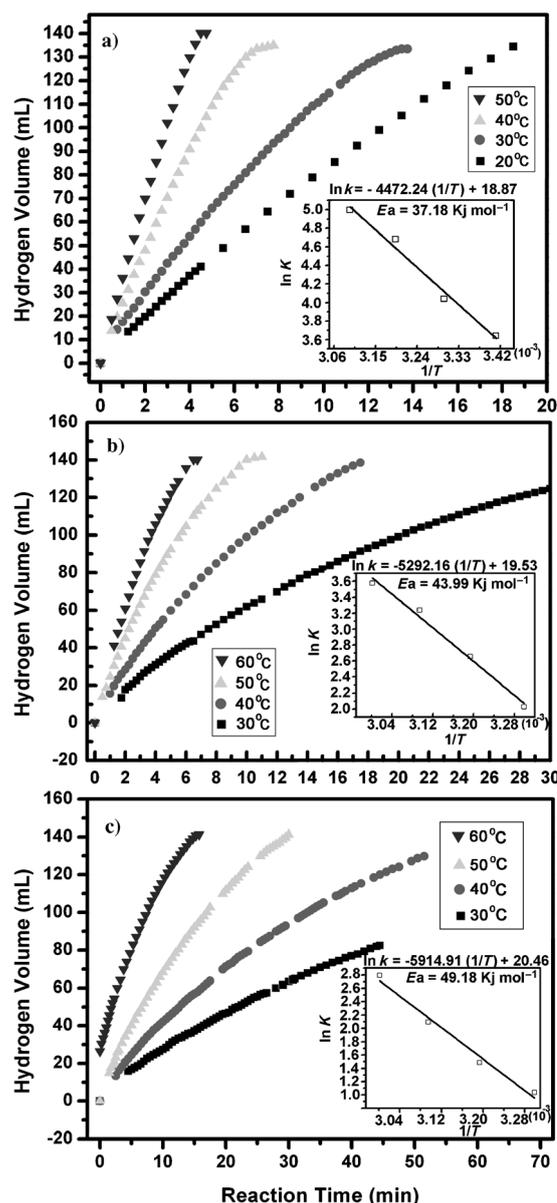
Figure 5. Plots of hydrogen production versus time during AB hydrolysis at different temperatures for a)  $\text{Ni}_{0.74}\text{Ru}_{0.26}$  alloy NPs; b) Ni@Ru core-shell NPs; c) monometallic Ru NPs. Insets show the reaction's Arrhenius plot in each case.
