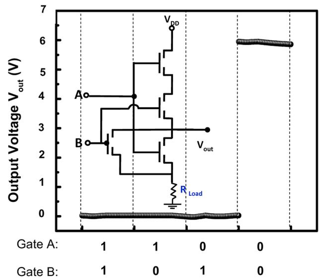
FIG. 3. Output characteristics of a NOR gate with resistive load using four hybrid ambipolar TFT. The supply voltage for the circuit is  $V_{DD} = 3$  V. Input voltages of 3 and  $-3$  V are treated as logics “1” and “0,” respectively.
