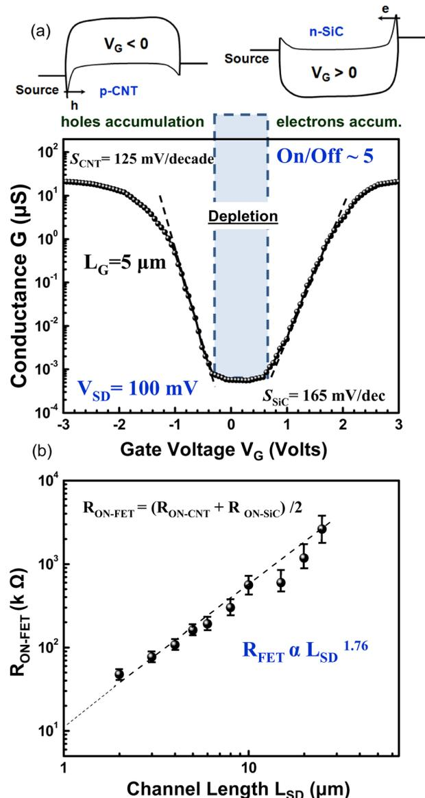
FIG. 2. (a) Electrical resistance measurements on devices with a channel width of  $50\ \mu\text{m}$  and channel lengths ranging from 2 to  $30\ \mu\text{m}$ . (b) Transfer characteristics (conductance  $G$  versus gate voltage  $V_G$ ) of the hybrid TFT having a  $L_{SD}$  of  $5\ \mu\text{m}$ .
