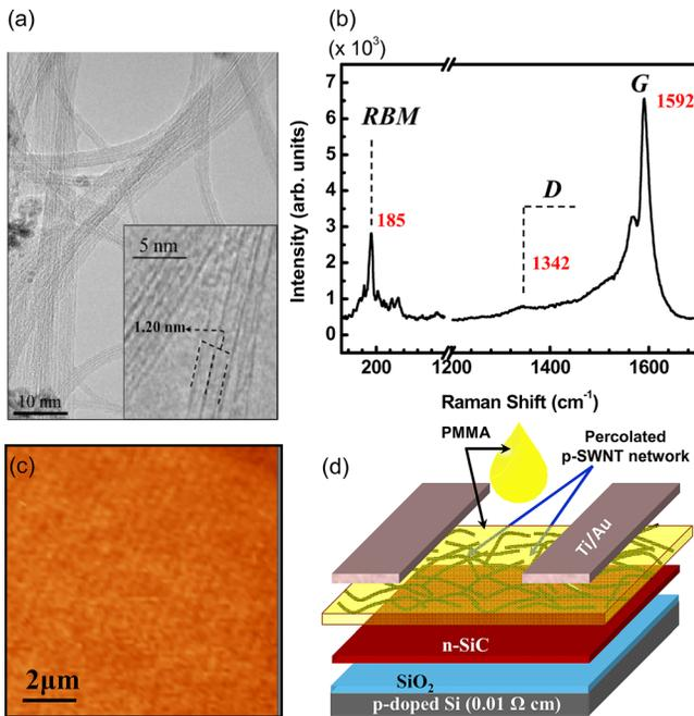
FIG. 1. (a) Representative TEM images of the purified SWNT. Inset is a close up view of a SWNTs bundle showing individual nanotube having a 1.2 nm-diam. (b) The corresponding microRaman spectrum. (c) Typical AFM image of the n-SiC surface, and (d) schematic of the hybrid n-SiC/p-SWNT back-gated TFT assembly.
